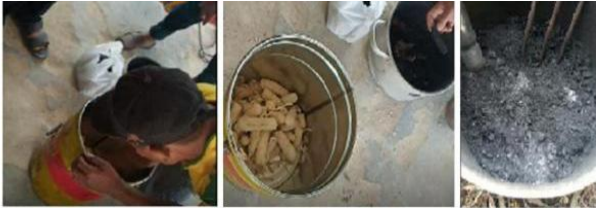
Figure 5. Production of Corn Cob Charcoal Through Pyrolysis.
