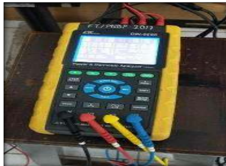
d. Pengujian alat power harmonic analyzer
